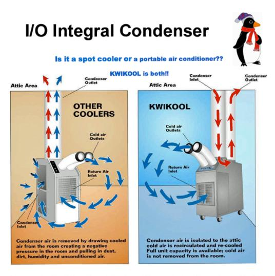
Many *spot coolers* claim to be portable air conditioners, but in fact they are not. To be an air conditioner, the condenser's inlet <u>MUST</u> be isolated from the conditioned space. In other words, if the unit only has one condenser duct (an outlet) then it is a spot cooler....not air conditioning!!
